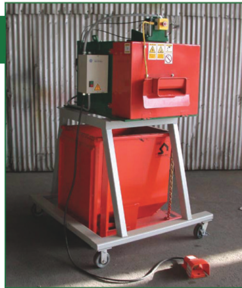
The Model 517 XHD is shown with an optional Easy Dump self-dumping hopper and hopper stand.
