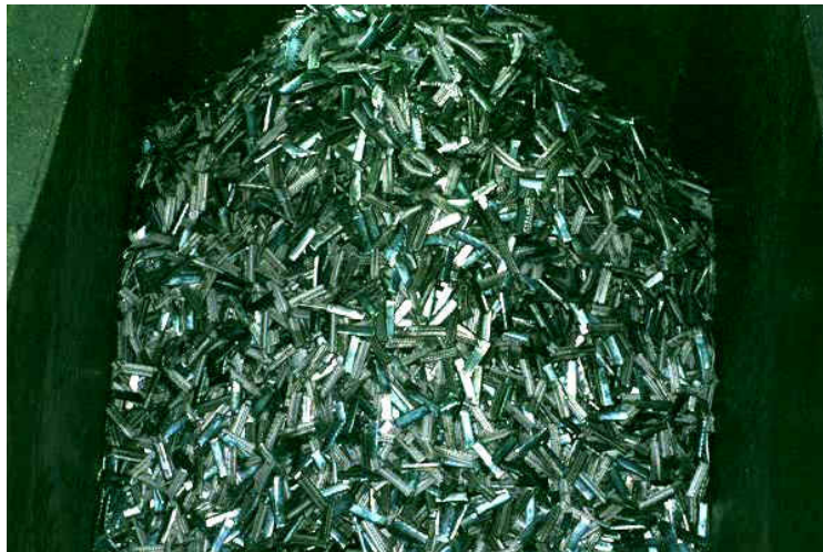
Scarf that has been processed through a Sweed chopper. The pieces are about 3" long.
