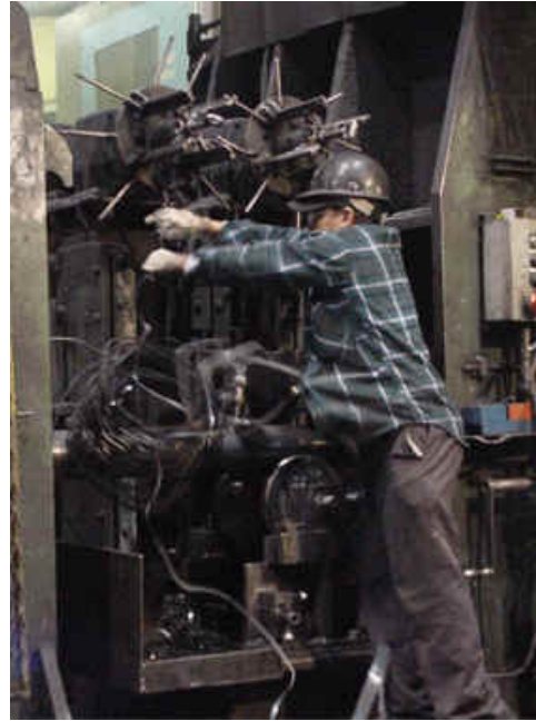
Typical "scarf ball" and mill operator "losing his shirt" to the scarf.
